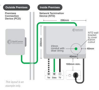
Indoor installation only. OptiComm equipment must be installed in a weather protected such as an enclosed garage or other location allowed under the cabling provider rules.
